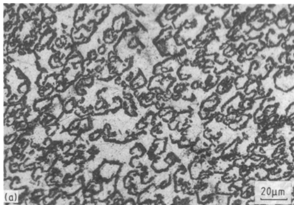
Figure 2 (a) Microstructure of specimen 5 representing nitridation mechanism ii with low conversion \alpha = 0.063 (optical micrograph, polished surface). (b) Microstructure of specimen 12 representing nitridation mechanism iii with controlled outward growth of a porous AlN/Al product and a local conversion of about \alpha \sim 0.5 (optical micrograph, polished surface). (c) Microstructure of specimen 17 representing nitridation mechanism iv with break-away nitridation and fully conversion \alpha = 1 (scanning electron micrograph, fracture surface).
